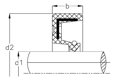
$\begin{array}{ll} b & = 7 \\ d1 & = 17 \\ d2 & = 28 \\ Material = NBR \end{array}$
